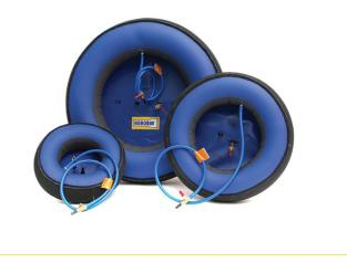
cell sealing surface, car wheel type - 1/4" BSP female valve for inflation and lever ball valve for rapid deflation. Pre-set relief valve to suit stopper size connected by 1200mm umbilical tube. Pull-out strap with hook and loop strip to attach U Gauge.
